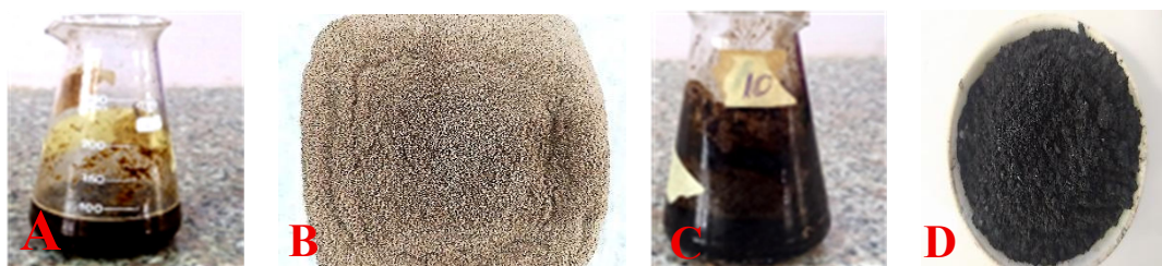
Figure 1 (a) Alkali treatment of Luffa cylindrica . (b) Sample A (c) Alkali treatment of Banana peel (d.) Sample B
