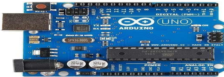
Figure 1: Diagram of an Arduino Board (Monk S., 2020)
