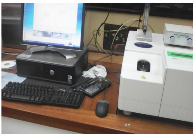
Figure 4: Photograph of FTIR equipment for the analysis of the compositions of the developed nanocomposites [29].
