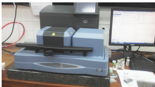
Figure 5: Photograph of DTA-TGA equipment for the analysis of the thermal properties of the developed nanocomposites[28].
