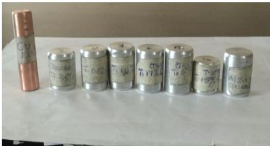
Figure 3: Developed beta-phase Titanium copper specimens and copper specimens (Udeh et al. , 2022)
