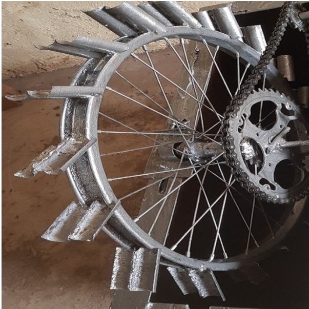
Fig 5: Constructed Rotor of the pelton wheel turbine
