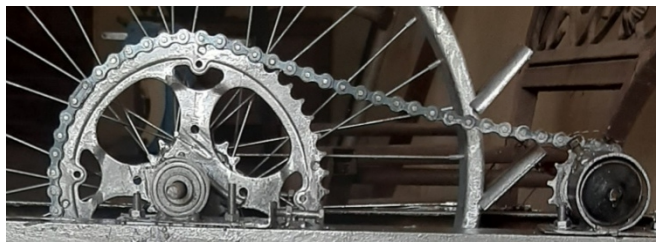
Fig 7: constructed chain and sprocket of the pelton wheel turbine
