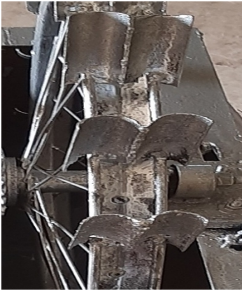
Fig 4:Constructed Bucket of the pelton wheel turbine
