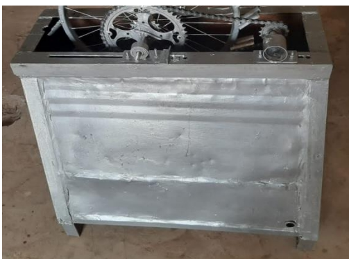
Fig 6: Constructed Housing of the pelton wheel turbine
