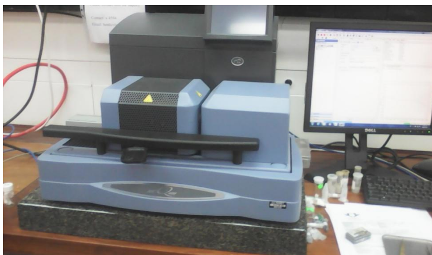
Figure 2: Photograph of DTA-TGA equipment. (STA Instruments).
